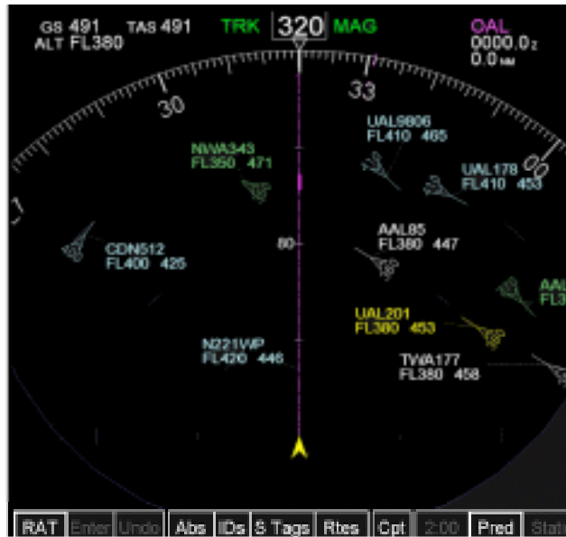
Figure 1. A snapshot illustration of the basic version of the Ames Flight Deck Display Research Group’s CDTI.
